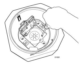
Unscrew the three Phillips screws located underneath the hinged door. Remove the inside portion of the back box.
